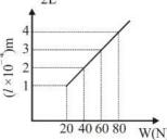
sectional area of the wire is  $10^{-6}$ m<sup>2</sup>, calculate the Young's modulus of the material of the wire
